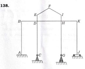
Neglecting axial deformation, the kinematic indeterminacy of the structure shown above is
